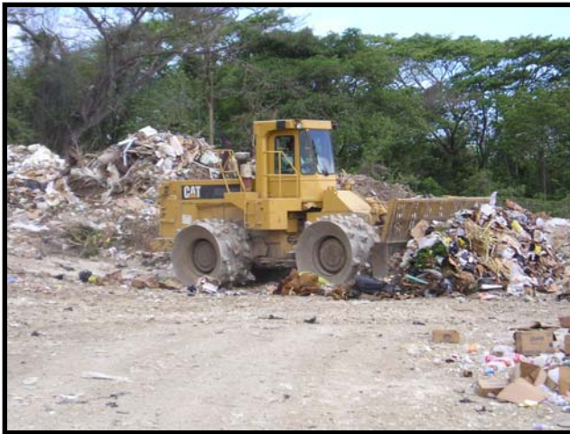
Acquisition of Landfill Equipment - Compactor
